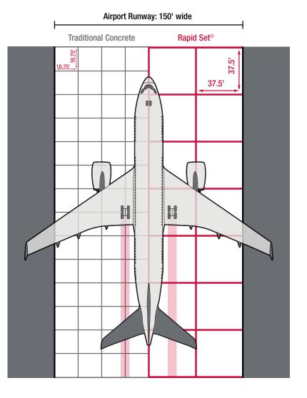
Most wide-bodied aircraft like the Boeing 787 Dreamliner have the outside tires within two feet of a longitudinal joint in a traditional pavement design. Since most concrete damage occurs on or near the joints, the current pavement design may not be conducive to long life. Using a larger slab made of Rapid Set Cement Concrete may alleviate this problem.
