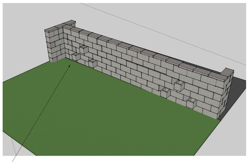
6x8 block is used on the base surface Six block high with Caps
